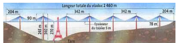
Figure 1 – Drawing showing a general overview of the bridge with corresponding dimensions ( http://www.animatif.com/ )
